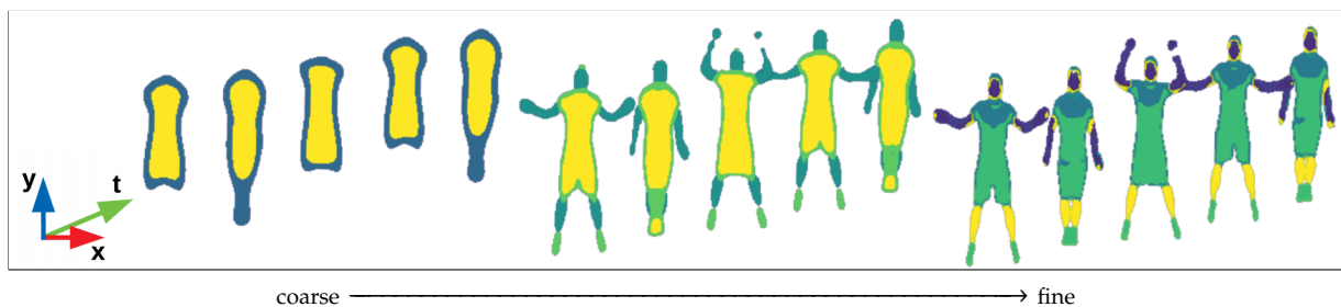
Figure 6.2: STVIs extracted at increasing spatial and temporal scales from a jumping-jack sequence. Note how finer scales capture more detail at the cost of temporal and spatial coherence, whereas coarser scales model more fundamental patterns. Two scales have been selected manually, the representation in the middle is achieved by automatic scale selection.
