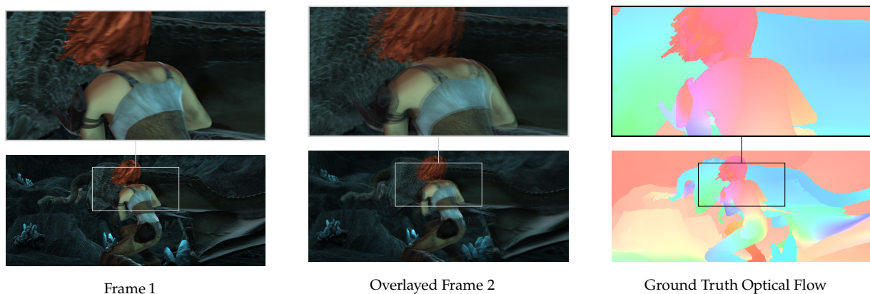
Figure 2.34: Two Frames from a Synthetic Video, and the optical flow between the two frames. Frame 1 is shown on the left, with Frame 2 overlaid on top of Frame 1 in the center. On the right the ground truth optical flow field is shown. The ground truth is available directly because the used dataset, Sintel [62], is synthetic.
